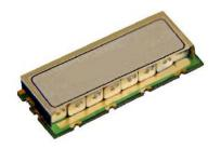
Ceramic monoblock filter, F0 2235MHz, bandwidth 4MHz, 40dB rejection.
