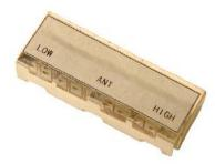
Ceramic monoblock duplexer, F0 1950MHz / 2140MHz, bandwidth 60MHz, 55dB rejection.
