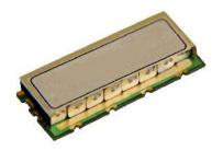
Ceramic monoblock filter, F0 1842.5MHz, bandwidth 225MHz, 19dB rejection.
