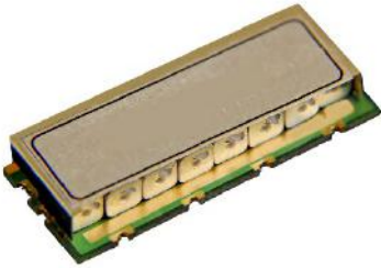
Ceramic monoblock filter, F0 1410MHz, bandwidth 110MHz, 40dB rejection.
