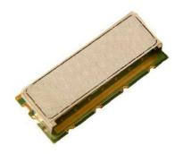
Ceramic monoblock duplexer, F0 897.5MHz / 942.5MHz, bandwidth 35MHz, 50dB rejection.
