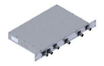
Same band combiner, diplexer, 900MHz same band combination. 880.1-889.9/925.1-934.1MHz and 902.5-914.9/947.5-959.9MHz, double unit 4-input / 2-output, 4.3-10 female, -155dBc, DC bypass for all ports, 19-inch cabinet installation.
