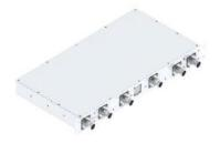
Same band combiner, diplexer, AWS systems combination. 1710-1720/2110-2120MHz and 1730-1755/2130-2155MHz, double unit 4-input / 2-output, 4.3-10 female, -155dBc, DC bypass for all ports, 19-inch rack installation.
