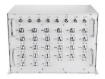
Multi-input multi-output combiner, point of interface, with the frequency band of 850/1800/2100/2300/2600MHz, 24-input / 4-output, used for passive DAS deployment, 7/16 DIN female, -150dBc.
