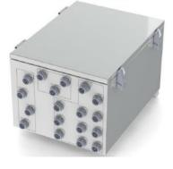
Multi-input multi-output combiner, point of interface, with the frequency band of 800/900/1800/2100/2300/2600MHz, 11-input / 4-output, used for passive DAS deployment, 7/16 DIN female, -150dBc, waterproof enclosure.
