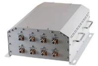
Multi-input multi-output combiner, point of interface, with the frequency band 800/900/1800/2100/2600MHz, 6-input / 1-output, used for passive DAS deployment, N female, -150dBc.
