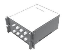
Multi-input multi-output combiner, point of interface, 900/1800/2100MHz, 6-input / 1-output, used for passive DAS deployment, N female, -150dBc.
