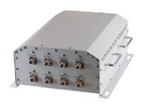
Multi-input multi-output combiner, point of interface, with the frequency band 800/900/1800/2100/2600MHz, 6-input / 1-output, used for passive DAS deployment, N female, -150dBc.
