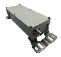
Interference mitigation filter with pass band 2600MHz FDD, single unit, 1-input / 1-output, 4.3-10 female, -155dBc, DC bypass.
