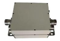
Interference mitigation filter with pass band 900MHz, double unit, 2-input / 2output, 4.3-10 female, -155dBc, DC bypass.
