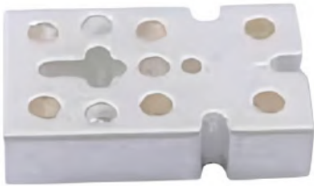
Ceramic waveguide filter, F0 3350MHz, bandwidth 100MHz, 30dB rejection.
