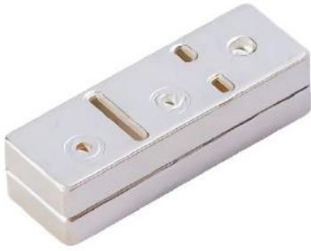
Ceramic waveguide filter, F0 2160MHz, bandwidth 20MHz, 42dB rejection.
