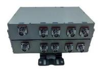
Multi-band RF combiner, pentaplexer, 694-806MHz and 824-894MHz and 1710-1755/2110-2155MHz and 1850-1990MHz and 2300-2700MHz combination, double unit 10-input / 2-output, 4.3-10 female, -155dBc, DC bypass for all ports.
