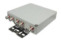
Multi-band RF combiner, pentaplexer, 694-803MHz/880-960MHz/1710-1880MHz/1920-2170MHz/2500-2700MHz combination, single unit 5-input / 1-output, 4.3-10 female, -155dBc, DC bypass for all ports.
