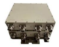
Multi-band RF combiner, quadplexer, 694-960MHz and 1710-1755/2110-2155MHz and 1850-1990MHz and 3300-3800MHz combination, double unit 8-input / 2-output, 4.3-10 female, -155dBc, DC bypass for all ports.
