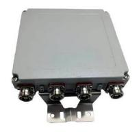
Multi-band RF combiner, quadplexer, 694-880MHz/890-960MHz/1710-1880MHz/1920-2700MHz combination, single unit 4-input / 1-output, 7/16 DIN female, -155dBc, DC bypass for all ports.
