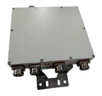
Multi-band RF combiner, quadplexer, 694-806MHz and 824-894MHz and 1710-1755/2110-2155MHz and 1850-1990MHz combination, single unit 4-input / 1-output, 7/16 DIN female, -155dBc, DC bypass for all ports.
