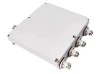
Multi-band RF combiner, quadplexer, 1710-1880MHz/1920-2170MHz/2300-2700MHz/3300-3800MHz combination, single unit 4-input / 1-output, 4.3-10 female, -155dBc, DC bypass for all ports.
