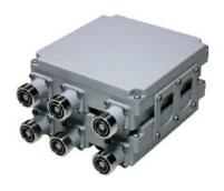
Multi-band RF combiner, triplexer, 694-806MHz/824-880MHz/890-960MHz combination, double unit 6-input / 2-output, 7/16 DIN female, -160dBc, DC bypass for all ports.
