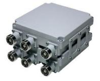
Multi-band RF combiner, triplexer, 694-960MHz/1710-1880MHz/1920-2170MHz combination, double unit 6-input / 2-output, 7/16 DIN female, -155dBc, DC bypass for all ports.
