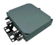
Multi-band RF combiner, triplexer, 1695-2700MHz / 3300-3800MHz / 5150-5925MHz, single unit 3-input / 1-output, 4.3-10 female, -155dBc, DC bypass for all ports.
