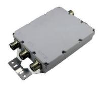
Multi-band RF combiner, triplexer, 380-862MHz/880-960MHz/1710-2700MHz, single unit 3-input / 1-output, 4.3-10 female, -155dBc, DC bypass for all ports.
