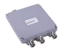
Multi-band RF combiner, triplexer, 612-960MHz/1695-2700MHz/3300-4200MHz combination, single unit 3-input / 1-output, 7/16 DIN female, -155dBc, DC bypass for all ports.
