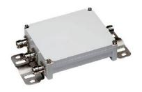
Multi-band RF combiner, triplexer, 1710-1880MHz/2300-2400MHz/2500-2700MHz, single unit 3-input / 1-output, 4.3-10 female, -160dBc, DC bypass for all ports.
