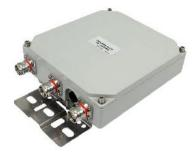
Multi-band RF combiner, triplexer, 2300-2400MHz and 2500-2570/2620-2690MHz and 2575-2615MHz, single unit 3-input / 1-output, 4.3-10 female, -160dBc, DC bypass for all ports.
