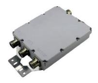
Multi-band RF combiner, triplexer, 1710-1755/2110-2155MHz and 1850-1990MHz and 2300-2700MHz combination, single unit 3-input / 1-output, 7/16 DIN female, -155dBc, DC bypass for all ports.
