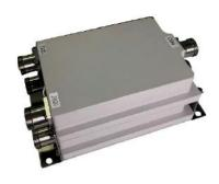
Multi-band RF combiner, diplexer, 1710-2170MHz/2300-2700MHz, double unit 4input / 2-output, 7/16 DIN female, -160dBc, DC bypass for all ports.
