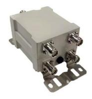
Multi-band RF combiner, diplexer, 2300-2400MHz/2500-2700MHz, double unit 4-input / 2-output, 7/16 DIN female, -160dBc, DC bypass for all ports.
