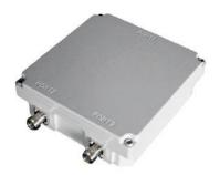
Multi-band RF combiner, diplexer, 824-880MHz/890-960MHz, single unit 2-input / 1-output, N female, -160dBc, DC bypass for all ports.
