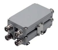
Multi-band RF combiner, diplexer, 380-2170MHz/2300-2700MHz, double unit 4-input / 2-output, 7/16 DIN female, -155dBc, DC bypass for high-band port.
