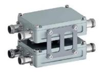
Multi-band RF combiner, diplexer, 1710-2170MHz/2300-2700MHz, double unit 4-input / 2-output, 7/16 DIN female, -155dBc, DC bypass for low-band port.
