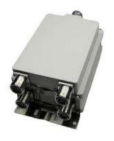
Multi-band RF combiner, diplexer, 617-803MHz/817-894MHz, double unit 4-input / 2-output, 7/16 DIN female, -155dBc, DC bypass for low-band port.
