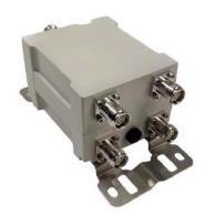
Multi-band RF combiner, diplexer, 1710-1880MHz/1920-2170MHz, double unit 4input / 2-output, 7/16 DIN female, -155dBc, DC bypass for all ports.
