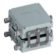
Multi-band RF combiner, diplexer, 1710-1755/2110-2155MHz and 1850-1990MHz, double unit 4-input / 2-output, 4.3-10 female, -155dBc, DC bypass for all ports.
