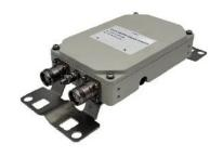
Multi-band RF combiner, diplexer, 380-960MHz/1710-2700MHz, single unit 2-input / 1-output, 4.3-10 female, -155dBc, DC bypass for all ports.
