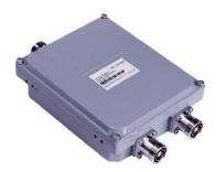
Multi-band RF combiner, diplexer, 694-746/824-894MHz and 758-798MHz, single unit 2-input / 1-output, 4.3-10 female, -155dBc, DC bypass for low-band port.
