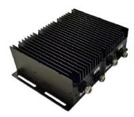
2-input / 1-output 3dB hybrid combiner is used for same band systems combination. This hybrid combiner covers the frequency band of 694-960MHz, with high isolation and low PIM performance. It is a double-unit mechanical design for 2T2R MIMO applications.
