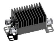
2-input / 1-output 3dB hybrid combiner is used for same band systems combination. This hybrid combiner covers the frequency band of 1710-2170MHz, with high isolation and low PIM performance.
