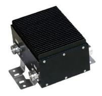
2-input / 1-output 3dB hybrid combiner is used for same band systems combination. This hybrid combiner covers the frequency band of 694-4200MHz, with high isolation and low PIM performance.
