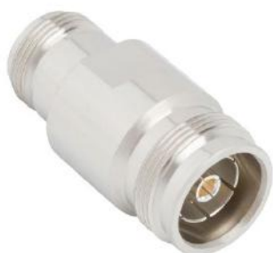
RF adaptor, 4.3-10 female (Jack) to N female (Jack), straight type.
