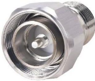
RF adaptor, 4.3-10 female (Jack) to 7/16 DIN male (Plug), straight type.
